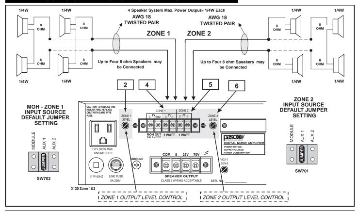
Fig. 26 - Rear Panel Zone 1 and 2 Speaker Connection Diagram
